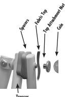
**5.** Unscrew top attachment nut from bolt. Place grommeted fabric top over the bolt, screw on top attachment nut and tighten until snug. Top should rotate easily - do not overtighten. Repeat this procedure on the remaining grommets.
