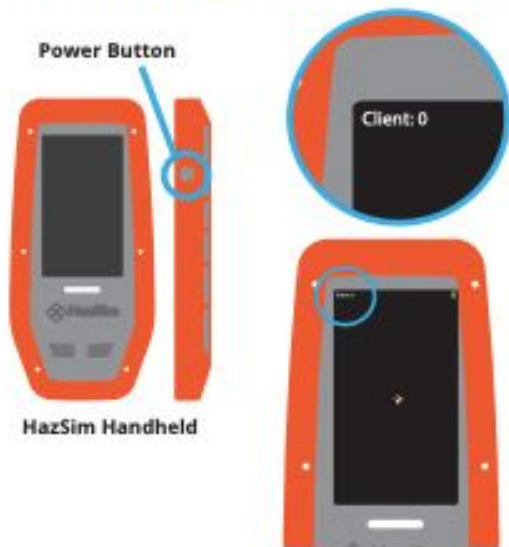
Figure 5: Power button for HazSim handheld.
