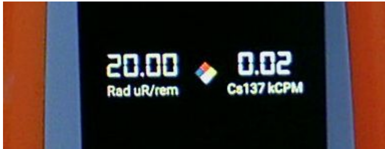
Figure 20: 'Calculated' meter displayed on HazSim for Cs137.
