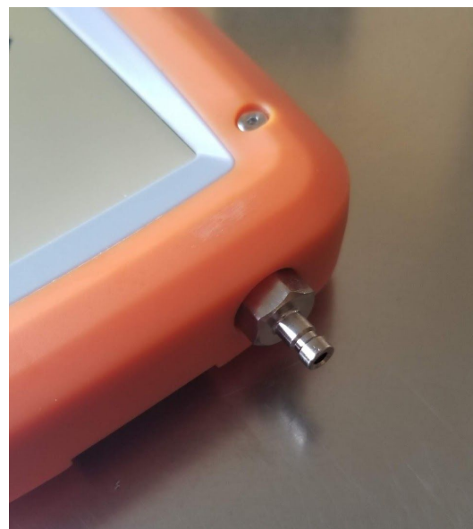
Figure 6: Confined Space Probe attachment point. Always remove probe for storage.
