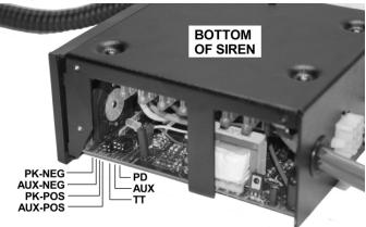
**Auxiliary Input Polarity** - The auxiliary input (green wire) is normally activated by applying a positive voltage to the wire. To activate it by connecting it to ground (negative), move the jumper from the "AUX-POS" pins to the "AUX-NEG" pins.
