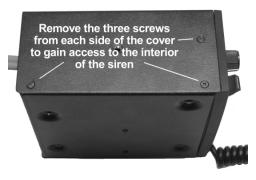
Cover Removal - Remove the three Philip head screws located on each side of the unit. DO NOT REMOVE THE SCREWS ON THE BOTTOM OF THE UNIT! Slide the top cover off of the unit. This cover can be removed completely from the siren unit. Carefully slide the cover off and set it aside.
