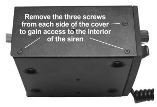
Cover Removal - Remove the three Philip head screws located on each side of the unit. DO NOT REMOVE THE SCREWS ON THE BOTTOM OF THE UNIT! Slide the top cover off of the unit. This cover can be removed completely from the siren unit. Carefully slide the cover off and set it aside.
