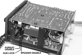
**Speaker Disable (Audible beep disable)** - The audible beep heard when the light control buttons on the siren are pressed can be disabled. If you move the Speaker Disable jumper from both pins onto only one pin, the audible beep will cease.
