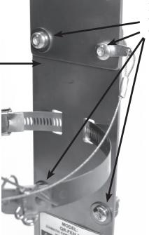
Mount at four points with Grade 5, 1/4" Type 4 hardware. WARNING: QM-FEH-1 is to be secured with a minimum of Grade 5, 1/4" Type 4 fasteners and washers. Failure to do so may result in non-compliance with safety standards.
